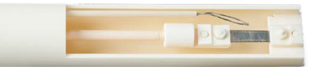
Tension sample holder kit made of alumina
