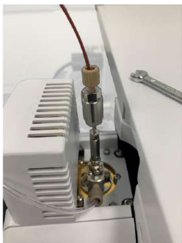
Figure 1: A ZORBAX Extend-C18, 80Å, 2.1 mm, 1.8 µm, 1200 bar pressure limit, UHPLC guard column was appended directly to the nebulizer to simulate the passing of a sample through a chromatographic column.
