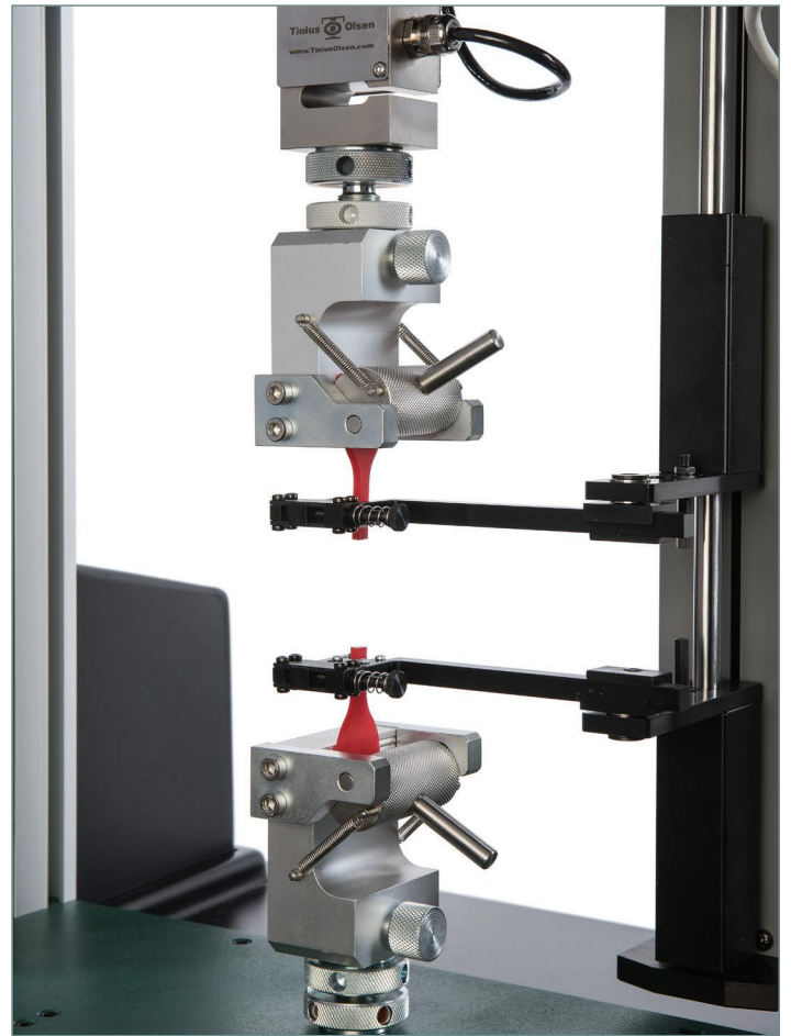
Model 100R long travel extensometer on specimen at specimen break.
