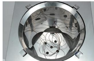
With the optional mounted sample temperature sensor, desired sample temperature can be precisely maintained to ensure thorough sterilization
