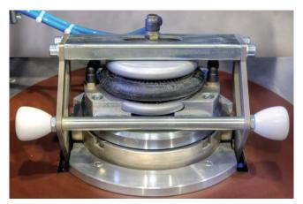
Pneumatic locking of the grinding vessel
