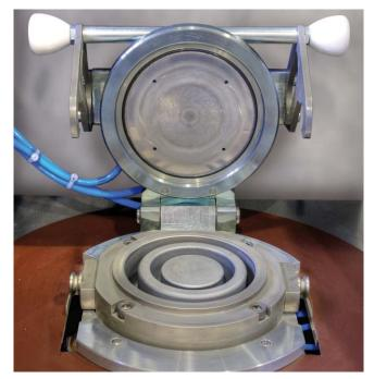
The grinding vessel can be opened with a handle
