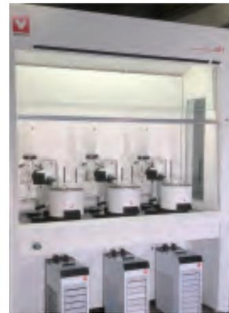
3 vertical type evaporators installed in a fume hood
