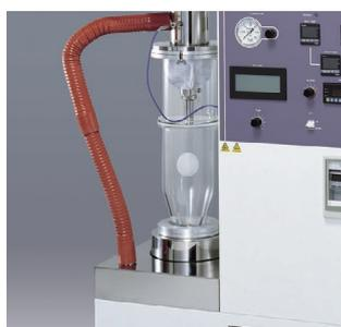
Use of the one touch removal system has made removal or cleaning of the drying chamber, cyclone or the product container much easier.
