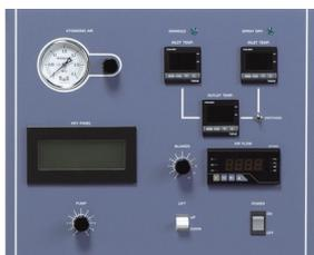
Inlet temperature, outlet temperature, and drying air amount are digitally displayed. Setting is made on the touch panel that allows operation settings, operation status displays as well as error display, and settings of various operation conditions. as well as error display, and settings of various operation conditions.
