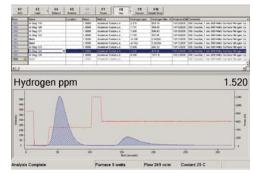
The advanced furnace control of the RHEN602 software facilitates the analysis of surface and bulk hydrogen in aluminum
