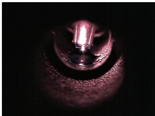
Tube-CAM simplifies method development and enables you to set the dispensing height and monitor the analysis.
